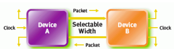
Figure 6 PCI-Express LVDS link (Source: PCISIG)
